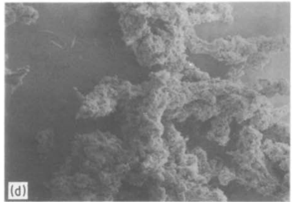
Figure 2 Natural rubber wear surfaces and debris as a function of frictional work input. (a, b) 2000 J m^{-2} , (c, d) 1350 J m^{-2} , (e, f) 690 J m^{-2} .
